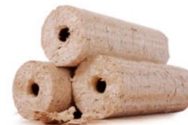
Natural firewood (left) is the best fuel for fireplaces, but you can also use wood-briquettes according to DIN EN ISO 17225-3, Class A1, length > 14 cm (5.51 in), diameter > 8 cm (3.15 in) (right).
