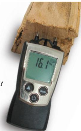
The water content in the wood can be quickly determined with a wood moisture meter.
